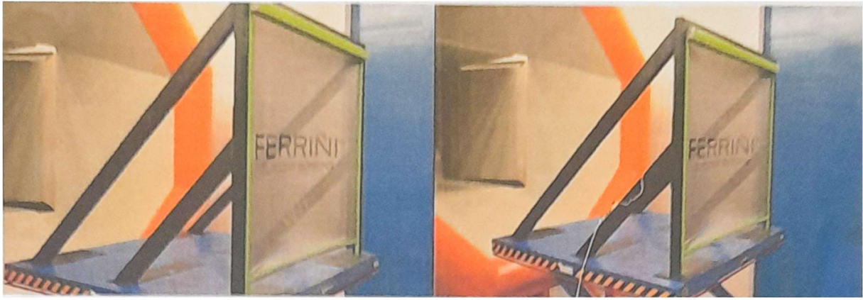
Figure 3: Zipline 105 (left) and Zipline Neo(right) under wind load .
